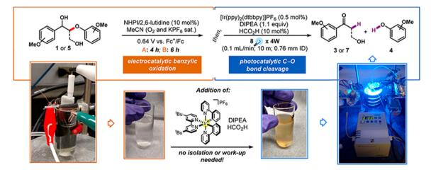
Fig. 11 Schematic for the one-pot electrocatalytic oxidation-reductive cleavage of  $\beta$ -O-4. Adapted from ref. 83 with permission from the American Chemical Society, copyright 2017.
