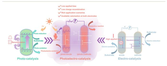
Fig. 2 Comparison of photo-, electro-, and photoelectro-catalysis.  $E_{FP}$  and  $E_{FN}$  are the quasi Fermi levels of holes and electrons, respectively;  $E_{Ox}$  and  $E_{Re}$  are the oxidative and reductive potentials of the substrate, respectively.
