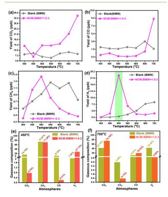
Fig. 4 Analytical results of GC: the yield of different gases from the blank sample and the mixed sample at different temperatures ((a) CO<sub>2</sub>; (b) CO; (c) CH<sub>4</sub>; (d) H<sub>2</sub>; (e) 450 °C; (f) 700 °C).
