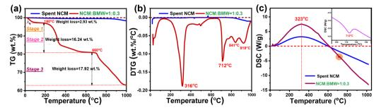
Fig. 3 The TG curve (a), DTG curve (b) and DSC curve (c) for cathode materials and roasting sample (heating rate -10 °C min<sup>-1</sup> and NCM: BMW = 1:0.3).
