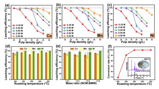
Fig. 7 Effects on the leaching efficiency of (a) Co, (b) Mn, (c) Ni (roasting temperature = 450 °C, NCM: BMW = 1:0.3, retention time = 15 min, leaching temperature = 50 °C, leaching time = 30 min), (d) (NCM: BMW = 1:0.3) and (e) (roasting temperature = 450 °C) and conversion rate of (f) Li at different roasting temperatures.
