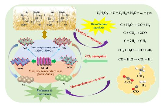
Fig. 8 Possible microthermal catalytic aerogenesis and metals conversion mechanism of BMW using waste NCM and its derivants as catalysts through thermochemical reactions.
