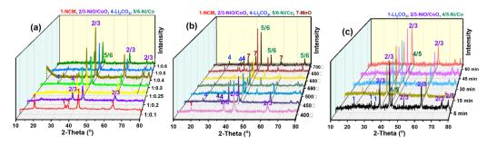
Fig. 2 The optimization of different parameters on the conversion of NCM into different products. (a) Effect of mass ratio of NCM: BMW (roasting temperature = 450 °C, retention time = 15 min); (b) effect of roasting reaction temperature (retention time = 15 min, NCM: BMW = 1:0.3) and (c) effect of retention time (NCM: BMW = 1:0.3, roasting temperature = 450 °C).
