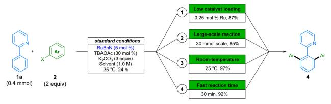
Scheme 6 Examples of targeted tuning of reaction conditions. Variations from standard conditions shown: (1) 2a, RuBnN (0.25 mol%), 70 °C, DMC; (2) 2b, 30 mmol scale, 4.5 h, 50 °C, DMC; (3) 2a, 25 °C, DMC; (4) 2a, 70 °C, DMC, 30 min. Yields are of isolated compounds.
