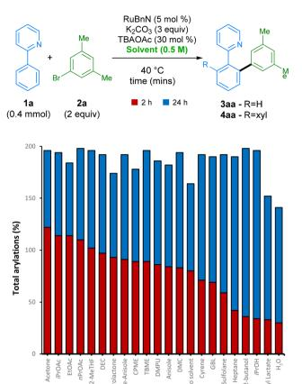
Scheme 2 Screen of green solvents at different reaction times. Yields were measured by GC-FID analysis of the crude reaction mixture using hexadecane as the internal standard. Solvent acronyms can be found in endnotes.<sup>46</sup>
