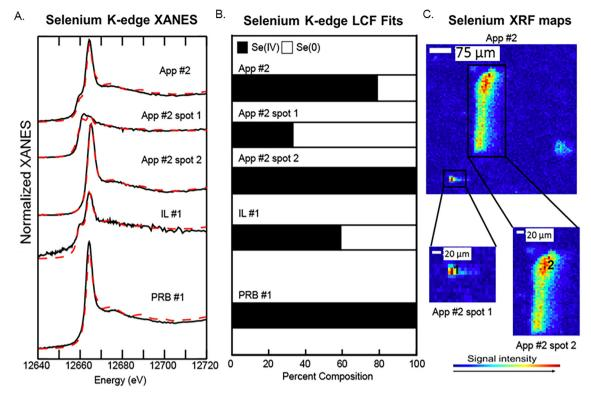
Fig. 5 Selenium speciation in fly ash samples analyzed by bulk and μ-XANES. A) Se-XANES spectra data (solid black lines) and model fits (red dotted lines) for bulk and microprobe analysis. B) LCF model results showing percent composition of Se for spectra collected by bulk and  $\mu$ -XANES. C)  $\mu$ -XRF maps of Se showing spots analyzed by  $\mu$ -XANES.
