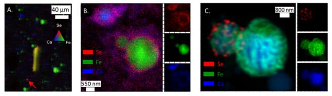
Fig. 3 (A) µ-XRF analysis of App #2 fly ash showing Se associated with Fe-rich fly ash particle (yielding yellow color) as well as single spots with intense Se red signal (see arrow); (B) nano-XRF analysis of App #1 (B) showing diffuse distribution of Se. This image shows the same portion of the sample as mapped in Fig. 2B; (C) nano-XRF analysis of PRB #1 fly ash showing discrete Se particles about 100-500 nm on a Fe-coated Ca-rich sphere.
