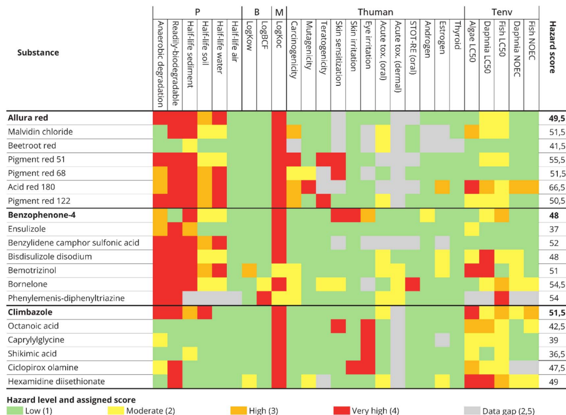
Fig. 4 Heat map and total hazard score of the three case-study chemicals and their potential alternatives for the P (persistence), B (bio-accumulation), M (mobility), human toxicity ( T_{human} ) and ecotoxicity ( T_{env} ) endpoints. The thresholds for the colour codes were based on ref. 34 and the scores were based on ref. 25. Colour codes indicate whether a hazard criterion is exceeded according to current regulatory standards and a very high hazard (red) is assigned. When hazard criteria fell below regulatory standards a high (orange), moderate (yellow) or low (green) hazard level is assigned. Chemicals with lower hazard scores compared to the case-study chemical are potentially safer alternatives.
