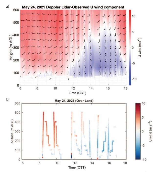
Fig. 5 Time—height cross section of the u (zonal) wind component from (a) the Doppler-lidar-observed horizontal winds (in m s<sup>-1</sup>), overlaid with horizontal wind barbs (in knots) plotted from 22 May 2021. Wind barbs are thinned by a factor of 5 in the time dimension and a factor of 2 in the height dimension to aid readability and (b) RAAVEN platform observations collected over land on May 24, 2021.
