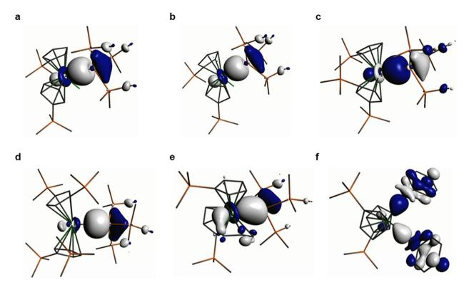
Fig. 3 Kohn-Sham Highest Occupied Molecular Orbitals (HOMOs) representing the M-Si or M-C σ-bonds in 1-6. (a) 1 (-4.866 eV); (b) 2 (-4.919 eV); (c) 3 (-4.884 eV); (d) 4 (-4.616 eV); (e) 5 (-4.571 eV); (f) 6 (-4.800 eV). Hydrogen atoms are omitted for clarity.
