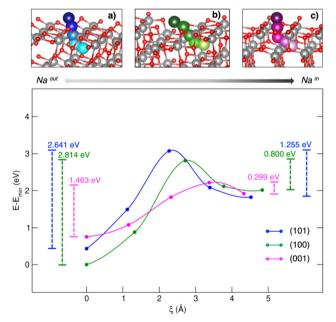
Fig. 2 Minimum energy paths (top) and corresponding energetics (bottom) for Na migration through the (a) (101)-, (b) (100)- and (c) (001)-TiO2 anatase surfaces. Energy barriers calculated from eqn (3) for the out/in migration are reported, respectively, at the left- and right-hand sides of the graph. Reproduced from ref. 91 [A. Massaro et al., Nanoscale Adv., 2020, 2, 2745] with permission from the Royal Society of Chemistry.91
