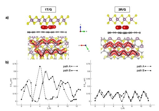
Fig. 1 (a) Side and top views of Na migration pathways through 1T- and 3R-MoS<sub>2</sub>/G interfaces; (b) corresponding energetics computed with the CI-NEB method at the PBE-D3BJ level of theory. Reproduced from ref. 76 [A. Massaro et al., J. Phys. Chem. C, 2021, 125, 2276–2286]. Copyright 2021 American Chemical Society.76
