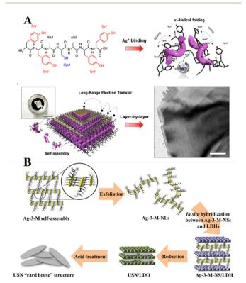
Fig. 10 (A) Schematics of the peptide-template-mediated formation of 2D Ag layers. 120 Reproduced with permission from ref. 120. Copyright © 2020 American Chemical Society. (B) Illustration of the formation process of single Ag layers within the interlayer space of LDH. Reproduced with permission from ref. 121. Copyright © 2019 American Chemical Society.
