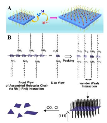
Fig. 5 (A) The illustration of the confinement growth of 2D Rh nanosheets at 120 °C for 6 h. Reproduced with permission from ref. 44. Copyright © 2016 American Chemical Society. (B) A possible growth mechanism of 2D Rh nanoplates proposed by Jang *et al.*  $^{36}$  Reproduced with permission from ref. 47. Copyright © 2010 American Chemical Society.
