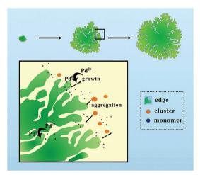
Fig. 6 A sketch of the mechanism of the formation of the 2D Pd dendritic nanostructures. Reproduced with permission from ref. 81. Copyright © 2014 The Royal Society of Chemistry.
