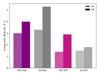
Fig. 6 Energy shifts ( $\delta E_{max}/\delta r$ ) in eV Å $^{-1}$  for K $\alpha$  (striped bars) and K $\beta$  (solid bars) spectra, calculated with RAS and 1-DFT BP86 for <sup>3</sup>MC and GS electron configurations.
