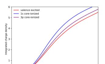
Fig. 8 Integrated RAS radial charge density (RCD) plots of the  $^3$ MC valence state, and the corresponding states with 1s and 3p holes calculated at the  $^3$ MC equilibrium geometry. To avoid effects of changes in core orbital occupation, only the Fe 3d  $^1$ 2g and  $^1$ 2g orbitals were included. Radial spin densities (RSD) for the same states are shown in Fig. S17 (ESI†).
