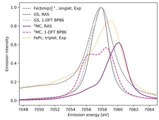
Fig. 2 Kβ X-ray emission spectra from experiment, <sup>18</sup> RAS and 1-DFT BP86 simulations. The simulated spectra for the electronic GS are calculated at the GS equilibrium geometry and the <sup>3</sup>MC spectra at the <sup>3</sup>MC equilibrium geometry.
