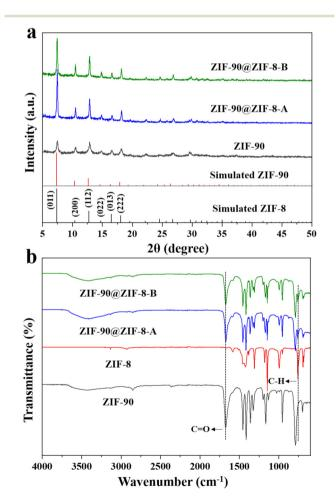
Fig. 3 (a) XRD spectra and (b) FTIR spectra of ZIF-90, ZIF-8, ZIF-90@ZIF-8-A and ZIF-90@ZIF-8-B.
