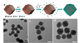
Fig. 6 (a) Schematic illustration of the synthesis of ZIF-90@ZIF-8-B. (b-d) TEM images of the intermediate sample collected during the synthesis of ZIF-90@ZIF-8-B at different reaction times of 2 min, 5 min and 20 min. The scale bar is 100 nm
