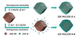
Fig. 1 Schematic illustration of the synthesis of ZIF-90@ZIF-8.
