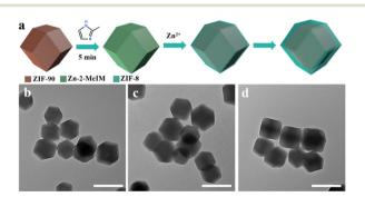
Fig. 4 (a) Schematic illustration of the synthesis of ZIF-90@ZIF-8-A. (b-d) TEM images of the intermediate sample collected during the synthesis of ZIF-90@ZIF-8-A at different reaction times of 2 min, 5 min and 20 min. The scale bar is 200 nm.
