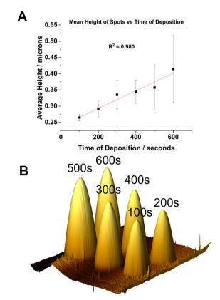
Fig. 4 Si-eATRP of Am at a SAM-functionalised gold electrode using [Am] = 10 wt% and [Cu<sup>II</sup>/TPMA] = 6.9 mM; (A) feature height as function of reaction time; (B) 3D representation of the AFM image of features deposited at  $E_{app} = -0.15 \text{ V}$  at increasing reaction times (100-600 s).
