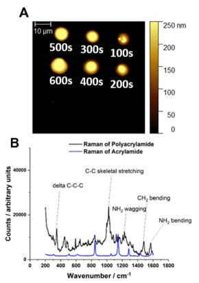
Fig. 2 For single-barrel SECCM eATRP of Am using [Am]: [HEBiB]: [Cu<sup>II</sup>]: [TPMA] = [20] : [1] : [0.5] : [0.625] at room temperature; (A) AFM image of the spots deposited at  $E_{\rm app}$  = -0.15 V; (B) Raman spectrum of PAm deposited during an extended TOD experiment (TOD = 1800 s;  $E_{app}$  = -0.15 V). Raman settings-exposure time: 600 s, laser:  $\lambda$  = 820 nm, power: 100%, objective: 50×, grating: 1200 l mm<sup>-1</sup>, pinhole: IN
