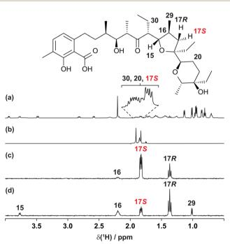
Fig. 1 (a) Conventional 600 MHz <sup>1</sup>H, (b) interferogram band-selective pure shift, (c) GEMSTONE CLIP-COSY and (d) GEMSTONE TOCSY NMR spectra of lasalocid in CDCl3. In (c) and (d) the transmitter frequency (indicated by the coloured label) was placed on the signal of proton 175. The CLIP-COSY mixing time  $(\tau_{\text{m}})$  in (c) was 120 ms, whilst the TOCSY mixing time in (d) was 30 ms. Full experimental details are provided in the
