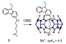
Fig. 2 (a) Design concept of a fluorescent receptor for anions with a 'turn-on' response. (b) Example of the supramolecular complexation of the pH probe in the cavity of cucurbit[6]uril.
