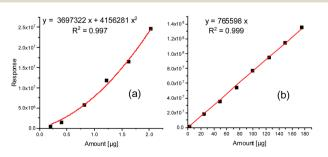
Fig. 2 Calibration curves of (a) MDI and (b) 1,4-butanediol (see the Experimental).
