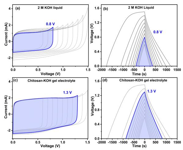
Fig. 7 (a) Cyclic voltammetry at  $0.1 \text{ mV s}^{-1}$ , (b) galvanostatic charge discharge at  $0.1 \text{ A g}^{-1}$  of activated carbon using liquid 2 M KOH from 0.6 to 1.5 V, (c) cyclic voltammetry at 0.1 mV s<sup>-1</sup> and (d) galvanostatic charge discharge at 0.1 A g<sup>-1</sup> using chitosan-KOH gel electrolyte
