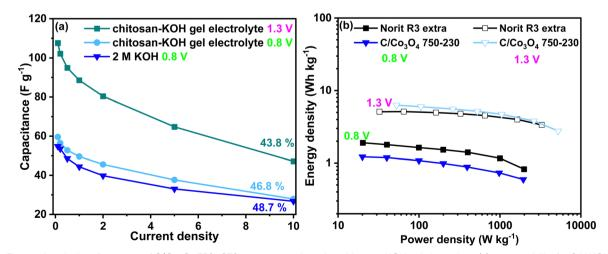
Fig. 10 Electrochemical performance of  $C/Co_3O_4$  750–230 nanocomposite using chitosan–KOH gel electrolyte: (a) rate capability for 2 M KOH at 0.8 V and for chitosan–KOH gel electrolyte at 0.8 and 1.3 V, (b) Ragone diagram of  $C/Co_3O_4$  750–230 nanocomposite and Norit R3 extra using 2 M KOH at 0.8 V and chitosan–KOH gel electrolyte at 1.3 V.
