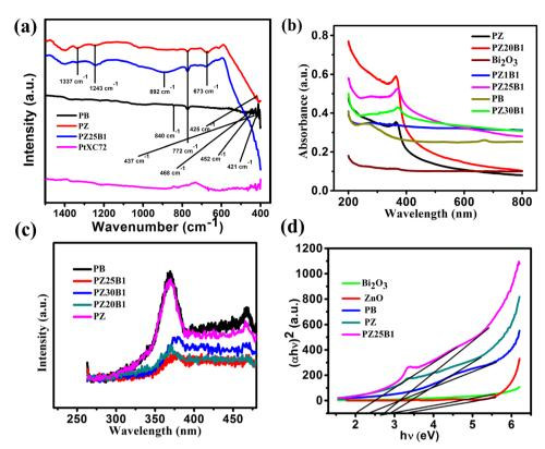
Fig. 5 (a) FTIR spectra of PB, PZ, PZ25B1, and PtXC72 catalysts (b) UV-Vis absorption spectra of synthesized catalysts. (c) The PL spectra PB, PZ, PZ5B1, PZ25B1 and PZ30B1. (d) The plot of  $(\alpha h \nu)^2$  versus  $h \nu$  for Bi<sub>2</sub>O<sub>3</sub>, ZnO, PB, PZ, and PZ25B1 nanocatalysts.
