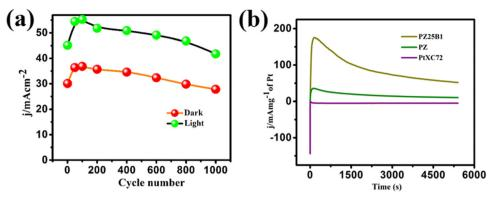
Fig. 9 (a) The long-term electrocatalytic stability of the PZ25B1 catalyst obtained from multiple cycling of voltammograms in both the presence and absence of visible light illumination in 0.5 M MeOH + 1 M NaOH solution at 50 mV s<sup>-1</sup> scan rate. (b) CA profiles of PtXC72, PZ and PZ25B1 electrodes at a fixed potential of -0.3 V up to 5400 s under the light.
