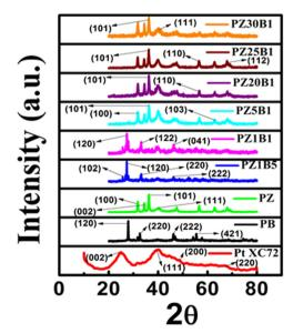
Fig. 1 (a) PXRD patterns of the synthesized Pt-Bi<sub>2</sub>O<sub>3</sub> (PB), Pt-ZnO (PZ) and various compositions of Pt-ZnO-Bi<sub>2</sub>O<sub>3</sub> (PZB) nanocatalysts.
