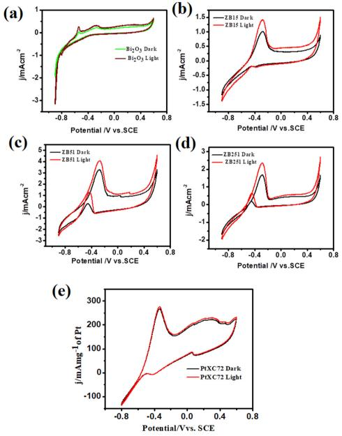
Fig. 6 Cyclic voltammograms of unplatinised supports in 0.5 M MeOH + 1 M NaOH solution at 25 °C (a)  $Bi_2O_3$  (b)  $ZnO: Bi_2O_3$  (1:5) (c)  $ZnO: Bi_2O_3$  (5:1) (d)  $ZnO: Bi_2O_3$  (25:1) with and without irradiation.
