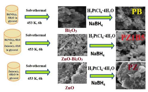
Scheme 1 The synthesis scheme of Pt-ZnO-Bi<sub>2</sub>O<sub>3</sub> heterojunction
