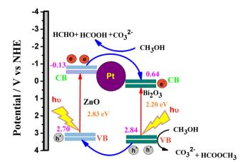
Fig. 12 Schematic mechanism of methanol photo-oxidation by Pt-ZnO-Bi<sub>2</sub>O<sub>3</sub> ternary catalyst
