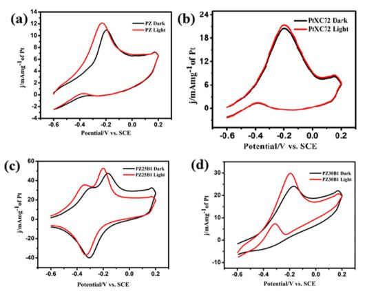
Fig. 10 CO oxidation of catalysts (a) PZ (b) PtXC72 (c) PZ25B1 (d) PZ30B1 with and without light irradiation in the 0.5 M NaOH solution using a scan rate of 50 mV s<sup>-1</sup> at 25 °C.
