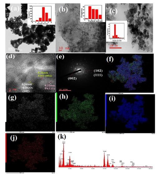
Fig. 3 TEM images (a) PB (b) PZ and (c) PZ25B1, (d) HRTEM images of PZ25B1, (e) SAED (f) elemental mapping (overlapping profiles) of PZ25B1 composite obtained from TEM, (g) mapping of O (h) Bi (i) Pt (j) Zn atoms (k) EDX from TEM, respectively.
