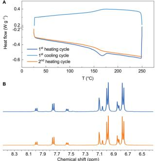
Fig. 1 (A) DSC characterization of derivative 7. (B) Details of the aromatic portion of the  ${}^{1}$ H NMR spectra in THF- $d_{8}$  of derivative **7** before (blue line) and after (orange line) the DSC thermal treatment.
