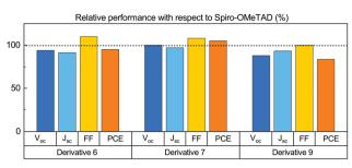
Fig. 3 Average  $V_{OC}$ ,  $J_{sc}$ , FF and PCE of PSCs prepared with derivatives 6, 7 and 9, with respect to the average values obtained for reference devices prepared using Spiro-OMeTAD as the HTL.
