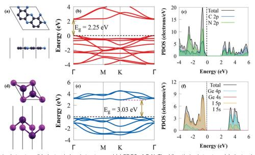
Fig. 1 The (a) optimised structure, (b) electronic band structure and (c) PDOS of C<sub>2</sub>N. The (d) optimised structure, (e) electronic band structure and (f) PDOS of the GeI2 monolayer. Ge, I, C and N atoms are denoted as magenta, purple, grey and blue balls, respectively. The Fermi energy level is set as 0 by the black dashed line.
