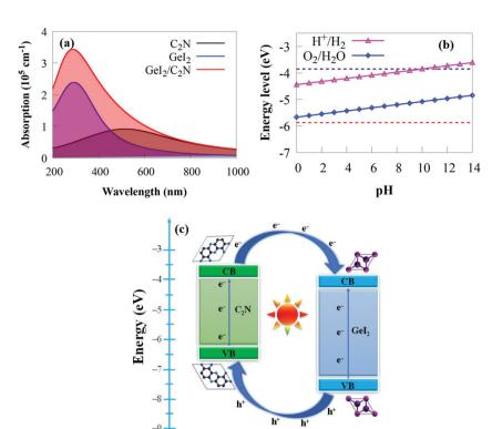
Fig. 6 (a) Calculated absorption spectra of the 2  $\times$  2 supercell of C<sub>2</sub>N, the 4  $\times$  4 supercell of Gel<sub>2</sub> and the Gel<sub>2</sub>/C<sub>2</sub>N vdW heterostructure. (b) The absolute energy bands for the conduction band minimum and valence band minimum of the  $Gel_2/C_2N$  vdW heterostructure with respect to pH (0-14). (c) Schematic diagram showing the transfer of photogenerated electrons and holes.
