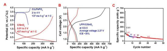
Fig. 6 Full cell analysis; C/LFP as the cathode and C/SnO<sub>2</sub> as the anode; (A) charge-discharge profile of C/LFP and C/SnO<sub>2</sub> at 1C in the half cell, (B) charge-discharge curve at C/2.5 and (C) rate capability curve of the full cell.
