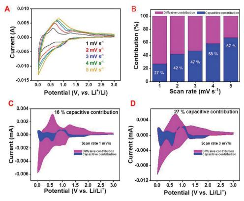
Fig. 4 Kinetics of the Li-ion in the C/SnO<sub>2</sub> composite; (A) cyclic voltammetry curve, (B) capacitive and diffusive contribution curve at different scan rates for a fixed potential (at 0.58 V), and capacitive and diffusive contribution in a cyclic voltammetry curve for a fixed scan rate, (C) 1 mV s<sup>-1</sup> and (D) 3 mV s<sup>-1</sup>.
