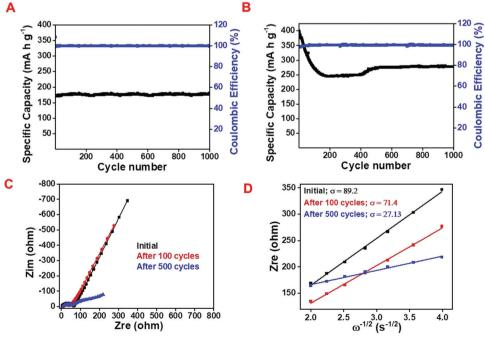
Fig. 5 Cyclic stability curve for (A) NAC at 200 mA  $g^{-1}$  and (B) C/SnO<sub>2</sub> at 375 mA h  $g^{-1}$ , (C) electrochemical impedance spectra (EIS) of C/SnO<sub>2</sub> at different stages of the cycles, (D) real impedance  $(Z_{rel})$  vs. angular frequency  $(\omega)$  plot where the slot refers to the Warburg impedance coefficient  $(\sigma)$ .
