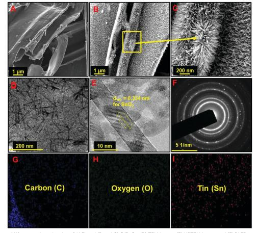
Fig. 1 FESEM images of (A) non-activated carbon (NAC) and (B and C) C/SnO<sub>2</sub>, (D) TEM image, (E) HRTEM image and (F) SAED pattern of C/SnO<sub>2</sub>, (F-I) Elemental area mapping of the C/SnO<sub>2</sub> composite from the TEM image.
