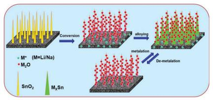
Scheme 2 Schematic presentation of the Li/Na-ion insertion and de-insertion reaction mechanism of the C/SnO<sub>2</sub> composite.
