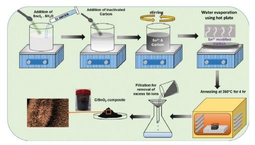
Scheme 1 Schematic presentation of the synthesis of the C/SnO<sub>2</sub> composite using the chemical dispersion method followed by annealing technique.
