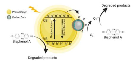
Graphical explanation of how CD assisted photocatalysis works for BPA degradation. Created with https://BioRender.com.
