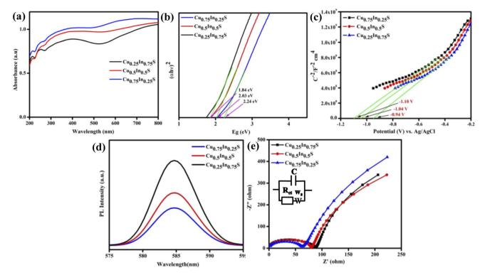
Fig. 2 Optoelectronic study of Cu<sub>0.25</sub>In<sub>0.75</sub>S (black line), Cu<sub>0.5</sub>In<sub>0.5</sub>S (red line), and Cu<sub>0.75</sub>In<sub>0.25</sub>S (blue line) QDs: (a) UV-Vis DRS spectra, (b) Tauc plot, (c) the M-S plot over a frequency of 1000 Hz in 0.1 M Na<sub>2</sub>SO<sub>4</sub>, (d) PL spectra, and (e) the EIS plot.
