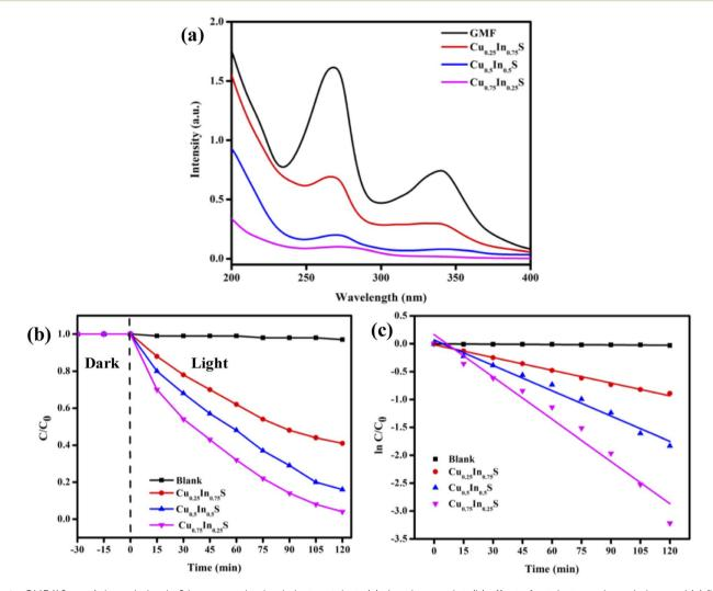
Fig. 4 GMF (10 ppm) degradation in 2 h over synthesized photocatalysts (a) absorbance plot, (b) effect of catalysts on degradation, and (c) fitted kinetic curve for the pseudo-first-order reaction.
