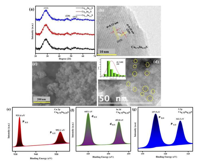
Fig. 1 Structural and compositional characterization: (a) XRD pattern of  $Cu_xIn_{1-x}S$  QDs with 3 different molar ratios 0.75 : 0.25, 0.50 : 0.50, and 0.25 : 0.75 of Cu : In, respectively (b) fringe pattern, (c) FESEM and (d) HRTEM images of  $Cu_{0.75}In_{0.25}S$  QD; (e) XPS analysis spectra of Cu 2p, (f) In 3d, and (g) S 2p elements in  $Cu_{0.75}In_{0.25}S$  QD.
