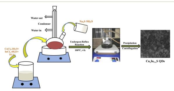
Scheme 1 Scheme for the synthesis of  $Cu_xIn_{1-x}S$  QDs by varying Cu: In molar ratios via the reflux strategy.
