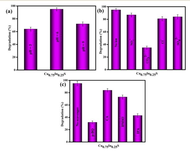
Fig. 5 Degradation efficiency of GMF over 10 ppm Cu<sub>0.75</sub>ln<sub>0.25</sub>S photocatalyst on different (a) pH solutions, (b) anions, and (c) scavengers.
