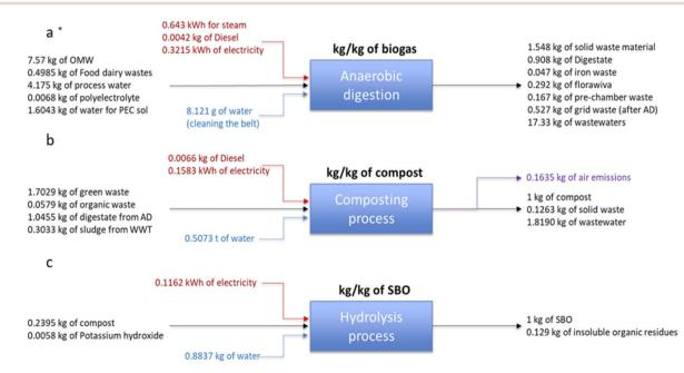
Fig. 12 Mass and energy input/output for the anaerobic digestion process in kg kg $^{-1}$  of biogas (a), composting process in kg kg $^{-1}$  of compost (b) and hydrolysis process in kg  $kg^{-1}$  of SBO (c). Legends: organic fraction of municipal solid waste (OMW); anaerobic digestion (AN); sludge waste water treatment section (WWT); soluble biobased product (SBO); insoluble organic residue accounted as unreacted compost.
