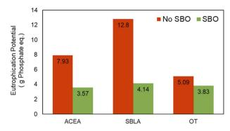
Fig. 15 Eutrophication potential (g phosphate eq.  $kg^{-1}$  biogas) for anaerobic digestion (AD) and compost processes without the addition of SBO ( $\blacksquare$ ) and with SBO addition ( $\blacksquare$ ). Legend: soluble biobased product (SBO).
