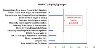
Fig. 13 Contribution of the global warming potential (GWP) of anaerobic digestion (AD) and compost plan.
