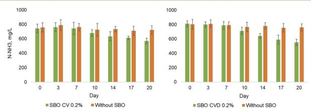
Fig. 5 Ammonia concentration in the presence and absence of 0.2% CV or CVD SBO during the trials of OT.
