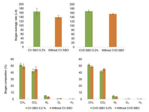
Calculated average production rate and composition of biogas over the whole duration of trials conducted in OT.
