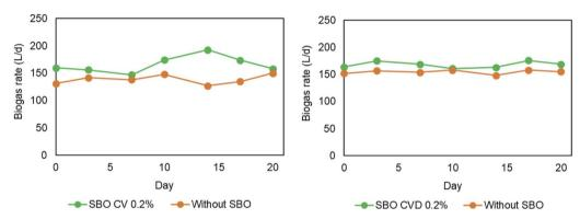
Biogas production rate over time in reactors A and B of OT in the presence and absence of CV SBO and CVD SBO, respectively.
