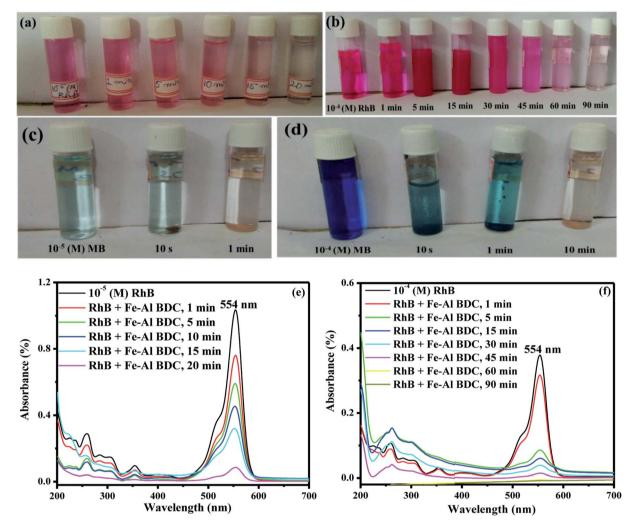
Fig. 6 Photographs of vials: (a)  $10^{-5}$  M RhB, (b)  $10^{-4}$  M RhB, (c)  $10^{-5}$  M MB, and (d)  $10^{-4}$  M MB. UV-vis spectral analysis of the photodegradation of (e)  $10^{-5}$  M RhB and (f)  $10^{-4}$  M RhB with a change in solar irradiation time for 0.10 g/100 mL Fe-Al BDC prepared at 473 K for 70 h at pH 7.
