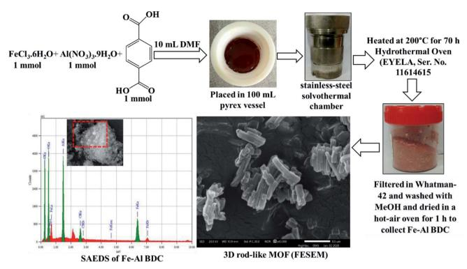
Fig. 1 Synthesis of the Fe-Al bimetallic 3D-rod-like MOF and FESEM and SAEDS studies after synthesis at 473 K for 70 h.
