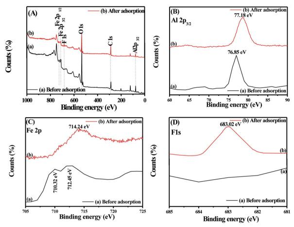
Fig. 9 XPS spectra of (A) (a) Fe-Al BDC prepared at 473 K for 70 h and (b) fluoride-adsorbed Fe-Al BDC prepared at 473 K for 70 h; (B) Al  $2p_{3/2}$  area analysis (a) before fluoride adsorption and (b) after fluoride adsorption; (C) Fe  $2p_{3/2}$  area analysis (a) before fluoride adsorption and (b) after fluoride adsorption and (D) F 1s area analysis (a) before fluoride adsorption and (b) after fluoride adsorption at pH 7.
