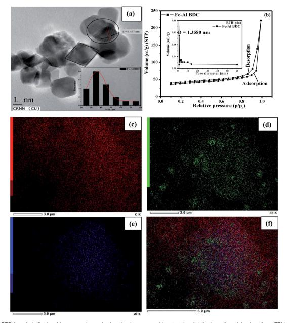
Fig. 3 (a) HRTEM analysis (lattice fringes are shown in the circular area, and inset - the distribution of particle sizes from TEM analysis), (b) nitrogen adsorption/desorption isotherm (inset - pore size distribution-BJH method), and elemental mapping showing (c) C, (d) Fe, and (e) Al and (f) overall elemental mapping in Fe-Al BDC prepared at 473 K for 70 h.
