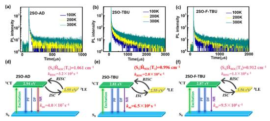
Fig. 3 Temperature-dependent transient PL spectra in doped films (doping concentration: 10 wt%) for (a) 2SO-AD, (b) 2SO-TBU and (c) 2SO-F-TBU. TADF kinetic rate constants, electronic energies and SOC matrix element values were obtained by theoretical calculations for (d) 2SO-AD, (e) 2SO-TBU and (f) 2SO-F-TBU
