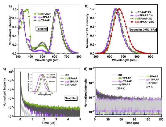
Fig. 4 (a) UV-Vis absorption and photoluminescence (PL) spectra of the dbfTPAAP, dpnTPAAP and dpTPAAP in dilute toluene (1  $\times$  10<sup>-4</sup> mol L<sup>-1</sup>). (b) Steady state PL spectra of the doped films with 3 wt% or 20 wt% in the DMIC-TRz matrix. Transient PL decay curves of these emitters (c) in neat films, inset: PL spectra in neat films, and (d) in the DMIC-TRz (3 wt%) matrix at different temperatures (under an argon atmosphere).
