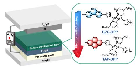
Fig. 1 Schematic illustration of the device architecture used in this study and chemical structures of BZC-DPP and TAP-DPP.
