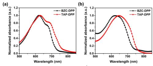
Fig. 2 UV-Vis absorption spectra of BZC-DPP and TAP-DPP in (a) solution (10<sup>-5</sup> M in chloroform) and (b) film state.
