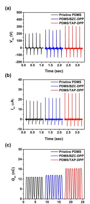
Fig. 5 Output characteristics of resulting TENG: (a)  $V_{\rm oc}$ , (b)  $I_{\rm sc}$ , and (c)  $Q_{\rm sc}$ .
