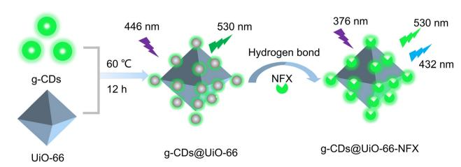
Scheme 1 Schematic representation for the preparation of g-CDs@UiO-66 and its application in norfloxacin sensing.
