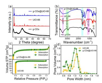
Fig. 2 (a) XRD patterns of the g-CDs (black line), UiO-66 (red line), and g-CDs@UiO-66 (blue line). (b) FT-IR spectra of the g-CDs, UiO-66, and g-CDs@UiO-66. (c) N2 adsorption-desorption isotherms, and (d) pore volume distributions of UiO-66 and g-CDs@UiO-66.
