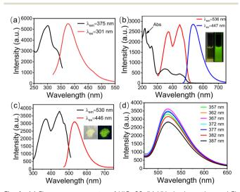
**Fig. 4** (a) Fluorescence spectra of UiO-66. (b) UV-vis absorption and FL spectra of g-CDs in aqueous solution. The inset shows a photograph of g-CDs under sunlight (Left) and UV light (Right). (c) FL spectra of g-CDs@UiO-66. The inset shows a photograph of g-CDs@UiO-66 under sunlight (Left) and UV light (Right). (d) g-CDs@UiO-66 emission spectra at different excitation wavelengths.
