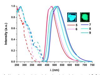
Fig. 4 Normalized excitation (—) and emission (—) spectra of **5–9** in 5 wt% PMMA films (right;  $\lambda_{\rm exc}$  = 340 nm). Pictures of **5** and **7** were taken under 365 nm light.
