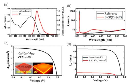
Fig. 13 (a) Absorbance and PL spectra of C-dots embedded in the PS solid matrix. (b) Experimental raw data of an absolute QY measurement. (c) The J-V curves for LSCs (100 cm<sup>2</sup>). (d) The J-V curves for standalone PVs and LSCs-PVs. Reproduced with permission from ref. 175. Copyright 2022, American Chemical Society.
