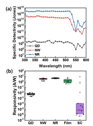
Fig. 7 (a) Specific detectivity of the CsPbBr<sub>3</sub> QDs, NWs, and NRs photodetectors at -3 V. (b) Responsivity of the CsPbBr<sub>3</sub> QDs, NWs, NRs, thinfilm, and single crystals (SCs) photodetectors.
