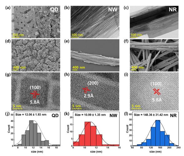
Fig. 2 TEM images of the CsPbBr<sub>3</sub> (a) QDs, (b) NWs, and (c) NRs. SEM images of the CsPbBr<sub>3</sub> (d) QDs, (e) NWs, and (f) NRs. HRTEM images with lattice fringes of the CsPbBr<sub>3</sub> (g) QDs, (h) NWs, and (i) NRs. Crystal size distribution histogram of the CsPbBr<sub>3</sub> (j) QDs, (k) NWs, and (l) NRs.
