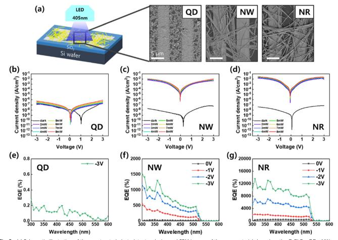
Fig. 5 (a) Schematic illustration of the constructed photodetector device and SEM images of the nanomaterials based on the CsPbBr<sub>3</sub> QDs, NWs, and NRs. J-V characteristics of the photodetectors under different illumination intensities based on the CsPbBr<sub>3</sub> (b) QDs, (c) NWs, and (d) NRs. EQE spectra of the photodetectors at various bias voltages based on the CsPbBr<sub>3</sub> (e) QDs, (f) NWs, and (g) NRs.
