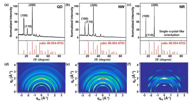
Fig. 3 XRD patterns of the CsPbBr<sub>3</sub> (a) QDs, (b) NWs, and (c) NRs with standard XRD reference (cubic: PDF 00-054-0752). 2D XRD patterns of the CsPbBr<sub>3</sub> (d) QDs, (e) NWs, and (f) NRs.
