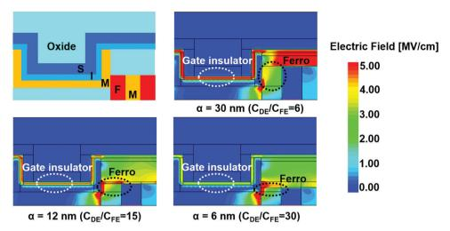
Fig. 6 Electric field profile of the 3D ferroelectric NAND flash cell during the program operation. The electric field profile of the 3D ferroelectric NAND flash cell according to the  $\alpha$  value (6, 12, 30 nm) during the program operation. The closer the color is displayed to red (blue), the stronger (weaker) the electric field intensity is. A decrease of  $\alpha$  leads to a weaker electric field across the gate insulator meaning reduced electrical stress on the gate insulator.
