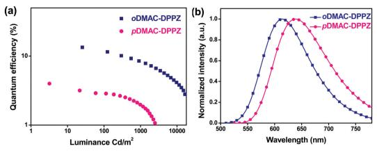
Fig. 5 (a) EQE-luminance characteristics, and (b) EL spectra of oDMAC-DPPZ- and pDMAC-DPPZ-doped OLEDs (1% doping concentration).
