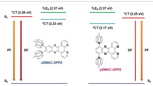
Fig. 3 Energy level diagram of oDMAC-DPPZ and pDMAC-DPPZ explaining the contribution of locally excited triplet state (3LEA) of DPPZ acceptor in the RISC process of the oDMAC-DPPZ TADF emitter.
