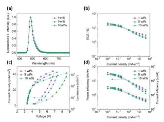
Fig. 4 OLED device performance for BOQAO. (a) Normalized electroluminescence spectrum. (b) EQE-current density curves. (c) Current density-voltage-luminescence curves. (d) Power efficiency-current density-current efficiency curves.
