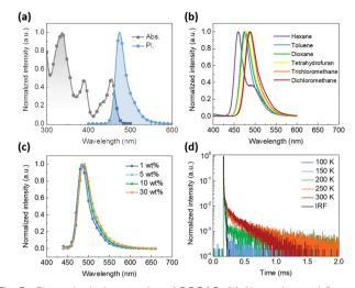
Fig. 3 Photophysical properties of BOQAO. (a) Absorption and fluorescence spectra of **BOQAO** in dilute toluene solution ( $10^{-5}$  mol L<sup>-1</sup>) at room temperature. (b) Fluorescence spectra of BOQAO in different solutions. (c) Fluorescence spectra of BOQAO in doped CBP films. (d) Transient spectra of 5 wt% BOQAO in CBP at different temperatures.
