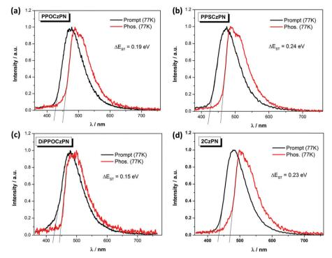
Fig. 5 Prompt fluorescence (at 77 K) and phosphorescence spectra (at 77 K) of (a) PPOCzPN, (b) PPSCzPN, (c) DiPPOCzPN, and (d) 2CzPN, in 10 wt% doped mCP thin films ( $\lambda_{exc}$  = 360 nm)
