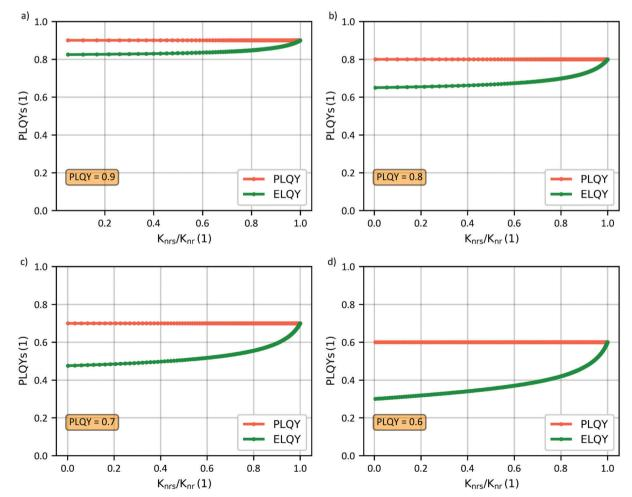
Fig. 2 For a fixed PLQY of 0.9 (a), 0.8 (b), 0.7 (c), 0.6 (d) the ELQY is calculated for all possible couples  $k_{nrs}-k_{nrt}$  which are solutions of eqn (1). In this calculation the other rates have been supposed known ( $k_f = 10^7 \text{ s}^{-1}$ ,  $k_{isc} = 10^7 \text{ s}^{-1}$  and  $k_{risc} = 10^6 \text{ s}^{-1}$ ).
