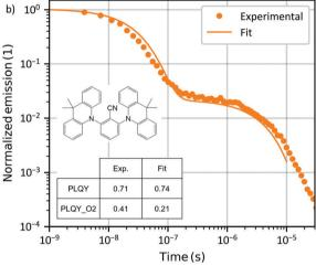
Fig. 4 Result of the global fit applied to two TADF films: 25ACA (a) and 26ACA (b). The experimental TrPL decay is shown with the resulting fit. The inset table indicates the experimental and fitted values for PLQY and  $PLQY_{O2}$ .
