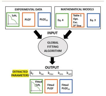
Fig. 3 The global fitting algorithm uses the parametrized mathematical model in order to minimize the difference between experimental (target) and fitted PLQY, PLQY\_O2 and TrPL data by adjusting the 5 excitonic parameters
