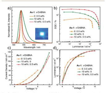
Fig. 6 (a) Normalized EL spectra, (b) EQE-luminance, (c) current densityvoltage, and (d) luminance-voltage characteristics of SP-OLEDs with different concentrations of Au-1 and v-DABNA. The image of the sensitized SP-OLED is shown in the inset of (a).
