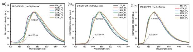
Fig. 5 The low-temperature and room-temperature PL of 2PO-2CF<sub>x</sub>Ph (a), 2PS-2CF<sub>x</sub>Ph (b) and 2AC-2CF<sub>x</sub>Ph (c) in Zeonex and the corresponding onsets of emission at 300 K.
