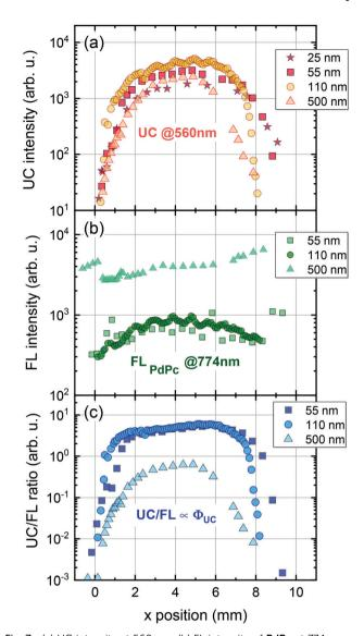
Fig. 7 (a) UC intensity at 560 nm, (b) FL intensity of PdPc at 774 nm and (c) UC/FL intensities ratio for different sensitizer layer thickness (indicated). Excitation, 730 nm. PdPc concentration in PS, 0.1 wt%. Each measurement was performed under the same conditions
