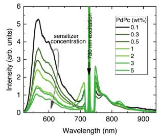
Fig. 5 UC emission spectra of PdPc/PS/Rub films with different PdPc concentrations. The spectra are normalized to the PdPc fluorescence maximum at 774 nm. Rub deposition conditions and PdPc-doped PS layer thickness (260 nm) were maintained the same. Excitation, 730 nm CW laser. A notch filter was used to suppress scattered excitation.
