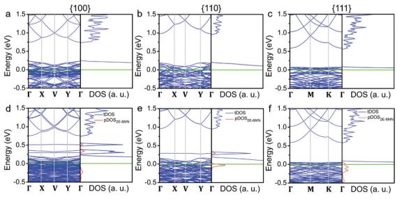
Fig. 8 (a-c) Band structures and density of states for the three different Cu<sub>2</sub>O crystallographic surfaces and (d-f) 2E-6MN-modified surfaces. Fermi level (green line) is set at zero in all band structures and density of states. The red peaks are the partial density of states (pDOS) from 2E-6MN molecules.
