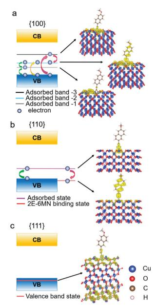
Fig. 9 Schematic illustration of the band diagrams and partial charge density distributions in real space for functionalized Cu<sub>2</sub>O (a) {100}, (b) {110}, and (c) {111} surfaces.
