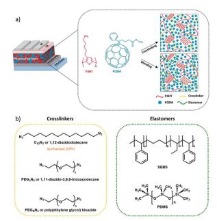
(a) Illustration of the strategies to improve the mechanical reliability of blend solar cells via fullerene cross-linking or elastomer blending. (b) Chemical structures of the cross-linker molecules and elastomers.
