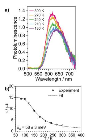
Fig. 6 Photoluminescence of 3 in polystyrene matrix at 0.1% (w/w). (a) steady state spectra recorded at temperatures from 300 to 180 K. (b) photoluminescence decay lifetime at temperatures from 300 to 80 K. showing the experimental data points and the best fit according to Egn (1).
