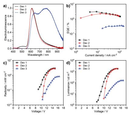
Fig. 9 Characteristics of devices 1-3: (a) electroluminescence spectra; (b) external quantum efficiency (EQE) vs. current density; (c) radiosity-voltage characteristics; (d) luminance-voltage characteristics.
