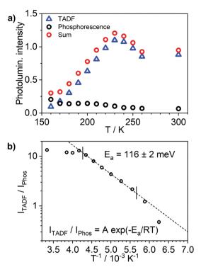
Fig. 4 Photoluminescence of complex 3 in toluene solution ( $c = 10^{-5}$  M) as a function of temperature: (a) intensity of TADF, intensity of phosphorescence and their sum (total intensity); (b) ratio of TADF to phosphorescence
