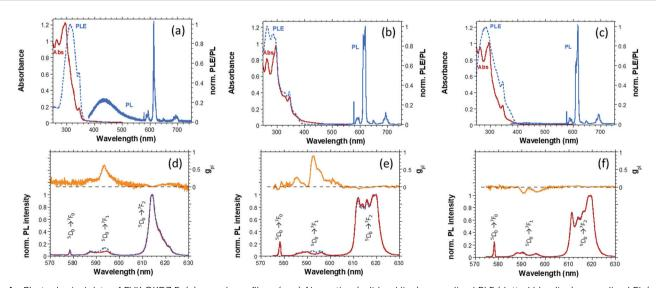
Fig. 1 Photophysical data of PVK:OXD7:Eu(III) complexes films: (a–c) Absorption (solid red line), normalized PLE (dotted blue line), normalized PL (solid blue line), (d–f) CP–PL for the two polarizations (solid red and dashed blue lines) and  $g_{pl}$  (orange line) of films embedding (*S,S*) **Eu1** (a,d), (*S,S*) **Eu2** (b,e) and (*S,S*) **Eu3** (c,f).  $\lambda_{ex}$  = 350 nm;  $\lambda_{em}$  = 614 nm (a),  $\lambda_{em}$  = 619 nm (b,c).
