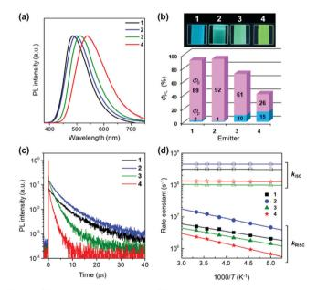
Fig. 5 (a) Steady-state PL spectra, (b) PL images and fractional quantum yields for prompt and delayed fluorescence ( $\Phi_{\rm p}$  and  $\Phi_{\rm d}$ ), and (c) transient PL decay profiles of  ${\bf 1-4}$  in the neat films measured at 300 K under N<sub>2</sub>. (d) Arrhenius plots of  $k_{\rm ISC}$  and  $k_{\rm RISC}$ , measured for the neat films of  ${\bf 1-4}$ , where the solid lines denote the least-squares fittings.
