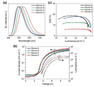
Fig. 6 (a) EL spectra, (b) current density-voltage-luminance (J-V-L)characteristics, and (c) EQE vs. L plots of the non-doped TADF-OLEDs based on 1-4 (Devices A-D).
