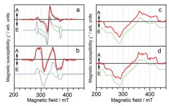
Fig. 2 Transient EPR spectra for (a) **4Cz-IPN**, (b) **PXZ-TRZ**, (c) **Cz-T**, and (d) **PIC-TRZ** in toluene detected at 550 ns after a laser flash at 77 K (red solid lines). The dotted lines are the simulation spectra: green, SOC-induced polarization; blue, hyperfine coupling (HFC)-induced polarization; and black, SOC plus HFC-induced polarization. Reproduced with permission. <sup>51</sup> Copyright 2015, American Chemical Society.
