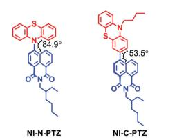
Fig. 6 Molecular structure of NI-N-PTZ, which shows TADF properties. The molecular structure of the reference compound NI-C-PTZ is also presented. Reproduced with permission.<sup>67</sup> Copyright 2019, American Chemical Society
