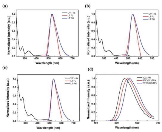
Fig. 2 Ultraviolet-visible and photoluminescence (PL) spectra of (a) 4CzTPN, (b) BTCz3CzTPN and (c) 2BTCz2CzTPN. (d) Room temperature fluorescence (RTFL) of 4CzTPN, BTCz3CzTPN and 2BTCz2CzTPN.
