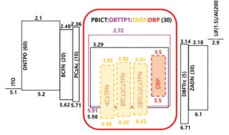
Fig. 5 Energy level diagram of the TADF-assisted hyperfluorescent devices.
