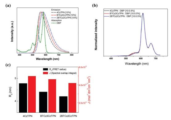
Fig. 7 (a) EL emission spectra of the assistant dopant at 10 wt% and UV-vis absorption spectra of DBP. (b) PL emission spectra of 10 wt% assistant dopant and 0.5 wt% DBP co-doped films. (c)  $R_0$  and J values of 4CzTPN, BTCz3CzTPN and 2BTCz2CzTPN.
