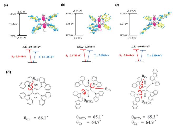
Fig. 1 Optimized ground state HOMO (blue) and LUMO (red) distribution and calculated energy details of (a) 4CzTPN, (b) BTCz3CzTPN and (c) 2BTCz2CzTPN. (d) Dihedral angles of the Cz and BTCz moieties in 4CzTPN, BTCz3CzTPN and 2BTCz2CzTPN.
