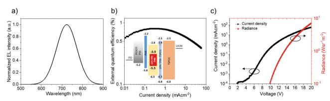
Fig. 5 Electroluminescence characteristics for the 15 wt% CAT-TPE device: (a) EL spectrum; (b) plot of EQE vs. current density with device structure schematic as inset; (c) plots of current density and radiance vs. voltage.
