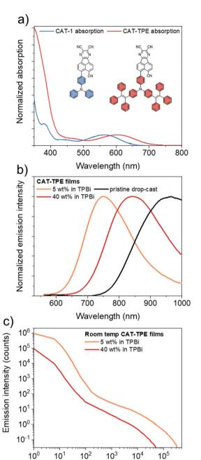
Fig. 2 (a) Absorption spectra of CAT-1 and CAT-TPE in toluene solution; (b) photoluminescence spectra of **CAT-TPE** films ( $\lambda_{exc}$  = 405 nm); (c) integrated photoluminescence kinetics of CAT-TPE films under vacuum ( $\lambda_{\text{exc}}$  = 400 nm, 10<sup>-5</sup> mbar).
