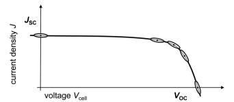
Fig. 5 Schematic of a JV curve with possible operating points for IS measurements,  $V_{\rm OC}$ ,  $J_{\rm SC}$  and MPP plus around the MPP. The points within the ellipses signify the essential steady-state operating point and the ellipses themselves indicate the range of voltage and current density that the devices undergo during the IS measurement, respectively.
