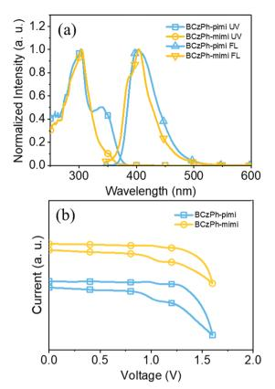
Fig. 2 (a) UV-Vis and fluorescence spectra and (b) cyclic voltammograms of BCzPh-pimi and BCzPh-mimi in toluene
