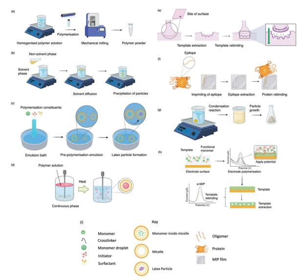
Fig. 2 Illustrative diagram depicting a range of different polymerisation techniques including: (a) bulk, (b) precipitation, (c) emulsion, (d) suspension, (e) surface, (f) epitope, (g) sol-gel, (h) electropolymerisation, and (i) each technique's associated key.
