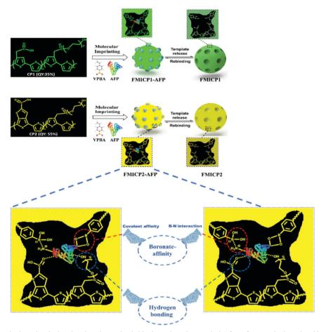
Fig. 7 A dual emission non-ionic molecular imprinted conjugated polythiophene-based paper device for α-fetoprotein detection. Mechanistic insight into dualemission conjugated polymers linked with boronate-affinity molecular imprinting technique. Reproduced with permission from ref. 180, Copyright 2020 Elsevier.
